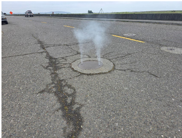
Figure 2: Smoke escaping the system through the pick holes of the Manhole
