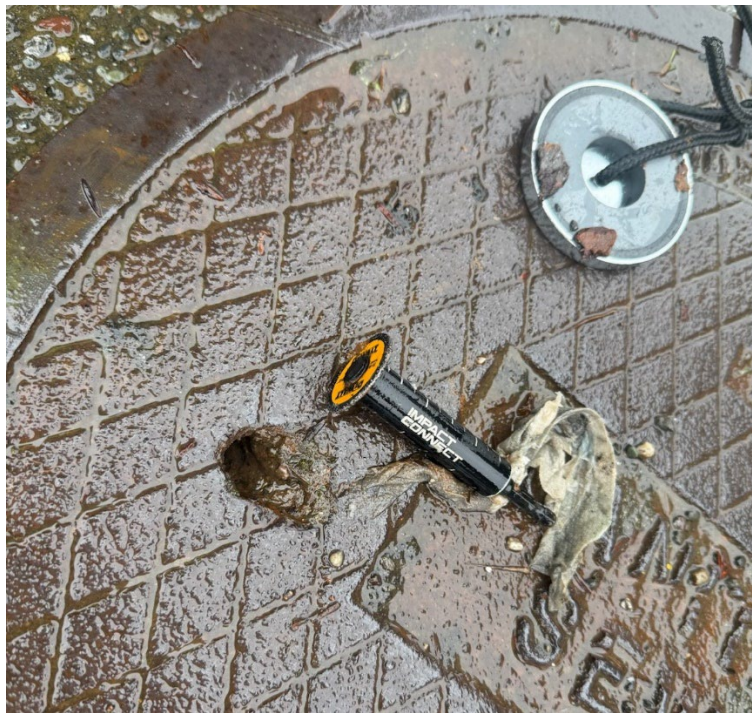
Figure 1: Impact Driver Pipe Cutting Tool recovered from Sewer Main
