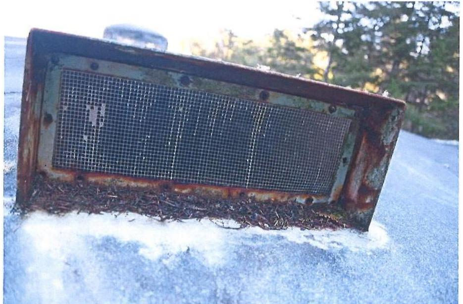
E-10 View of a cathodic protection handhole cover, illustrating severe corrosion at the circumference of the cover.
